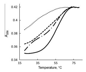
**Fig. 4.** Thermal melting profiles of RNA samples studied: wild type omega RNA, solid curve;  $3A \rightarrow 3C$  RNA, dashed curve;  $(A,U)_n \rightarrow (G,C)_n$  RNA, dotted curve;  $(CAA)_n \rightarrow U_{3n}$  RNA, dashed-dotted curve. The thermal melting experiments were performed in  $Mg^{2+}$ -free 10 mM sodium cacodylate buffer, pH 7.5, with 100 mM NaCl and 0.5 mM EDTA.
